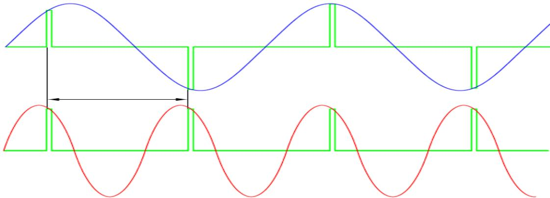
If the Doppler frequency produced by a moving target is exactly the same as the PRF ( $f_D = PRF$ ) then "sampling" occurs at the same point on each Doppler cycle. As far as the signal processor is concerned, it is as if the target were stationary. The same effect occurs if  $f_D$  is an integer multiple of PRF. Hence targets with certain radial velocities tend to be invisible to an MTI pulse radar.
